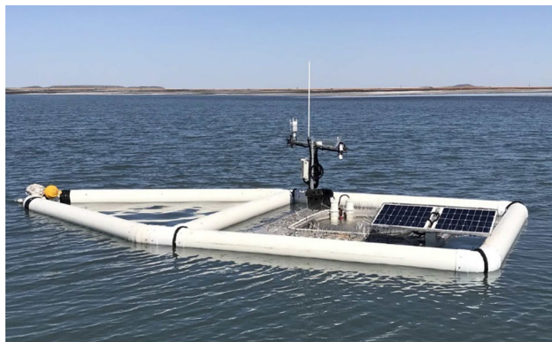
Fig. 2 Floating evaporation pan deployed on the open water area of the TSF
